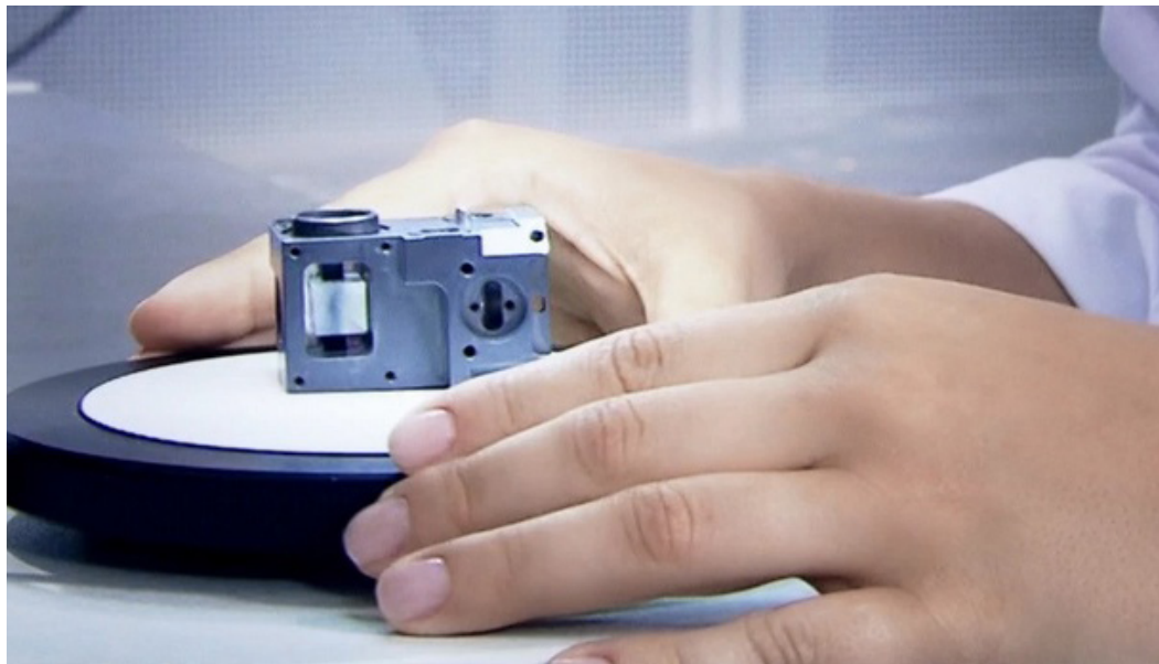
5 A gliding stage helps with positioning the sample – especially at high magnification levels.
