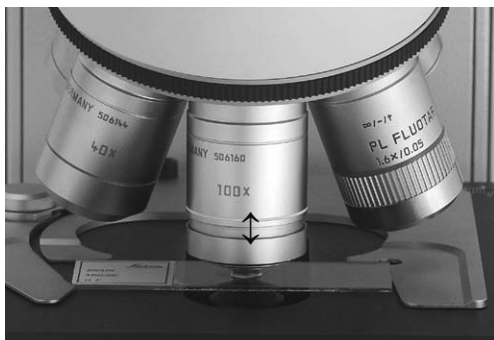
Fig. 63a Immersion objective, released
