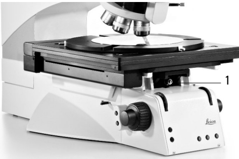
Fig. 32 Condenser height setting
