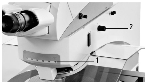
Fig. 40 LED status display
