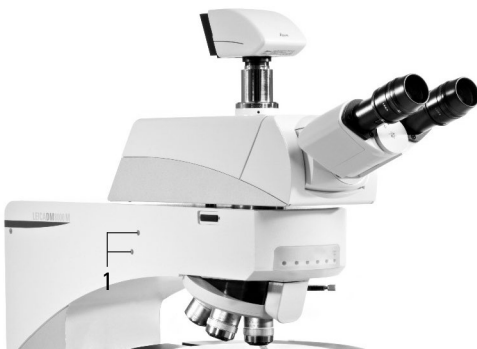
Fig. 30 Adjusting the aperture diaphragm in the reflected light axis
