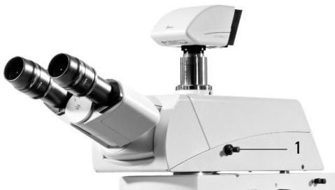
Fig. 43 Beam splitting on the tube 1 Control bar
