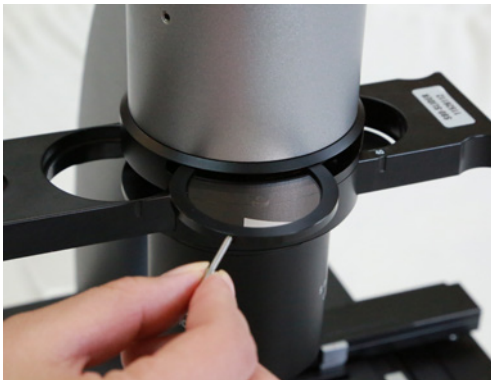
Fig. 9 Insert of transmitted light filter
