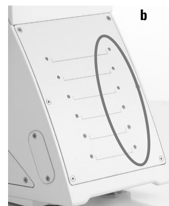
b Keypad for coded objective turret and coded reflector turret
