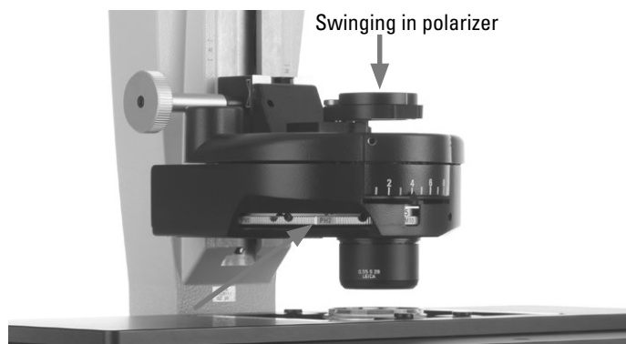
Condenser setting for tiltable transmitted light illuminator arm - configuring Wollaston prism
