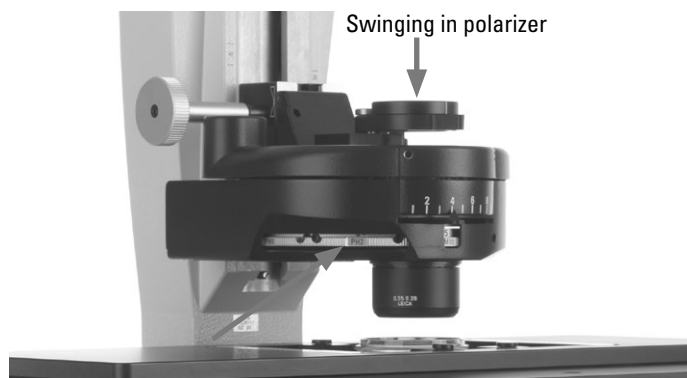
Condenser setting for tiltable transmitted light illuminator arm - configuring BF position
