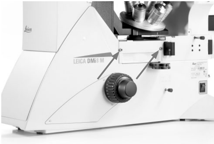
Screws for securing the reflector turret cover
