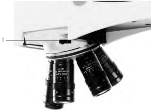
Fig. 55 Objective turret with objectives
