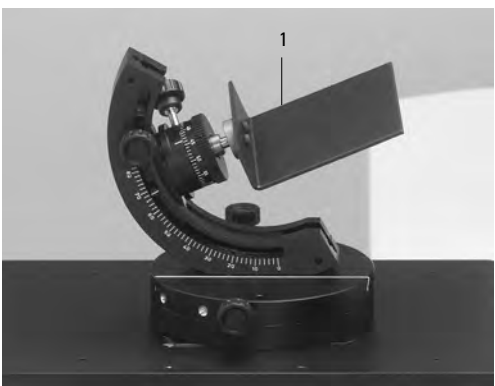
Fig. 45 Adjustable holder with receptacle for locking cylinders 1 Receptacle for locking cylinder
