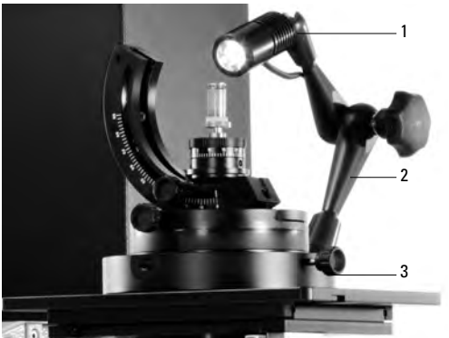
Fig. 4 Illumination equipment 1 LED spot illumination 2 Joint holder 3 Rotating mechanism
