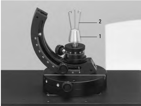
Fig. 43 Adjustable holder with shotgun shell casing holder 1 Shotgun shell casing 2 Conical base
