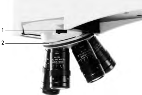
Fig. 5 Objective turret with objectives
