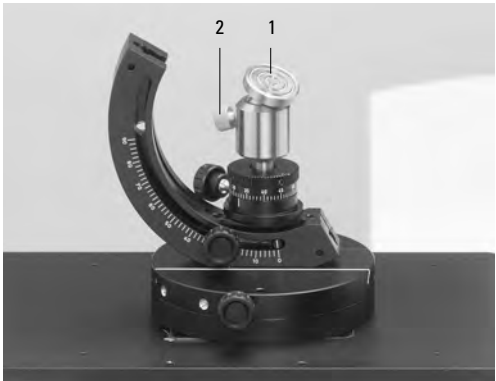
Fig. 48 Adjustable holder with Ø 25 mm stage with ball-and-socket joint
