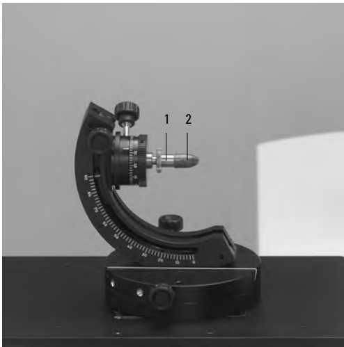
Fig. 38 Adjustable holder with paste-on cylinder for bullets
