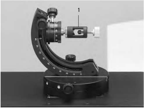
Fig. 45 Adjustable holder with receptacle for locking cylinders 1 Receptacle for locking cylinder
