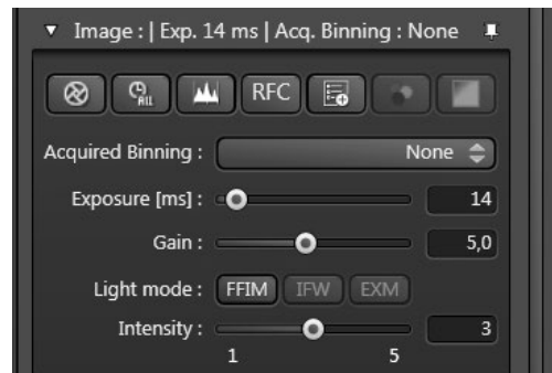
Fig. 5: Adjusting transmission for FFIM
