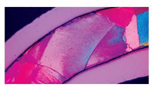
Copper core in spark plug electrode, etched with modified Adler's reagent. Viewed under polarised light at 50x magnification
