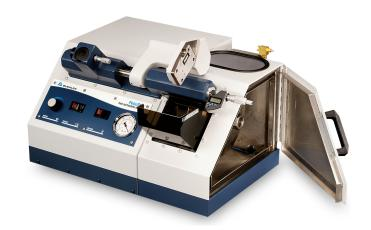
**Dimensions**: 23.5in [597mm] x 19in [483mm] x 16in [406mm] **Weight:** 94lbs [43kg]
