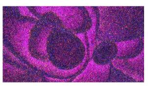
Additively manufactured AlSi10Mg electrolytically etched with Barker's reagent. Viewed under polarised light at 800x magnification
