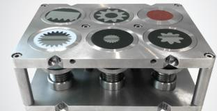
Self leveling vise for six round mounted samples up to 40mm (requires additional inserts). Incl. magnets.
