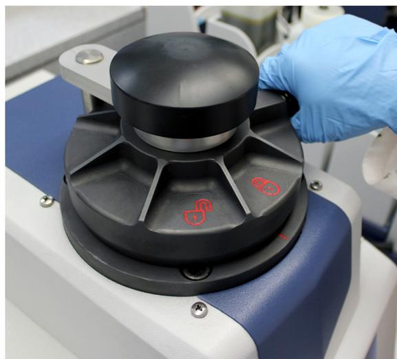
Compression mounting compounds utilize heat and pressure to encapsulate a specimen. Buehler's compounds minimize shrinkage while protecting and preserving sample edges during the preparation process.
