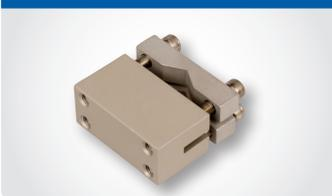
Small Double Saddle Chuck that securely holds specimen up to 0.875in [22mm] from 2 points
