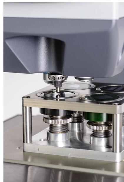
Please select the correct sample holder by sample diameter or a clamping device.
