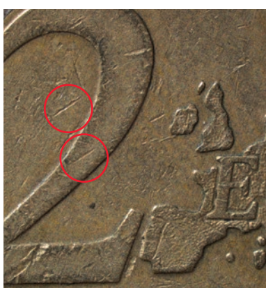
Leica LED3000 MCI: scratches become visible with the left illuminator arc
