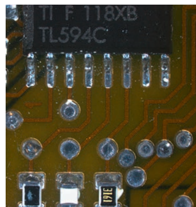
Leica LED3000 RL with crossed polarizers: reflections are almost completely eliminated – bad soldering can be seen easier
