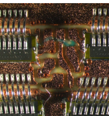
Leica LED3000 SLI: connecting wires on an electronics board highlighted by a side light
