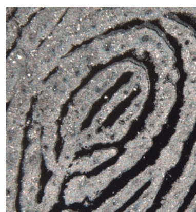
Leica LED5000 MCI: fingerprint on a CD in oblique light
