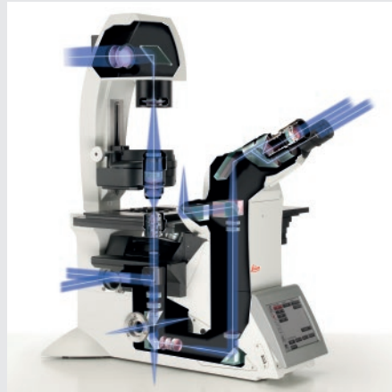
Opto-mechanical documentation of the Infinity Port
