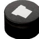
Graphite and mineral filled phenolic thermoset resin
