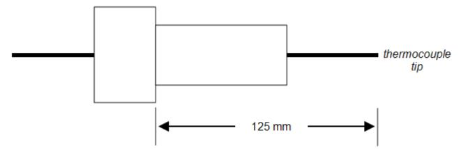
If thermocouples with different outer diameters are to be calibrated then end plugs with different size holes should be used. These may be ordered from Carbolite Gero. The maximum recommended diameter is 7.5 mm - larger diameters may experience too much heat conduction and give an incorrect calibration.
