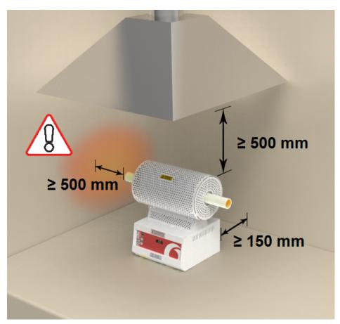
Depending on the application of the product, it may be appropriate to position it under an extraction hood. Ensure the extraction hood is switched on during use.
