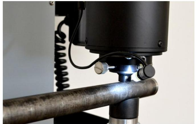
V Anvil standard and clamping device.
