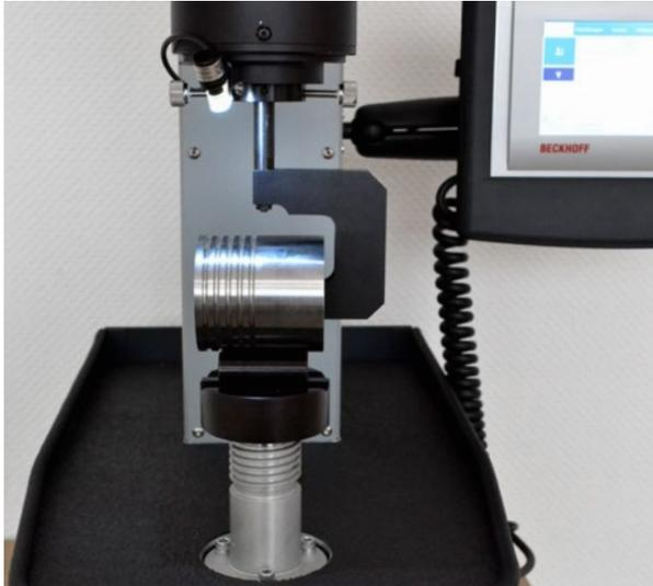
The Wilson RH2150 Rockwell hardness tester is the next generation Rockwell hardness tester.
