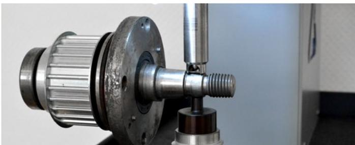
Anvil shallow, clamping device, indenter extension 2".
