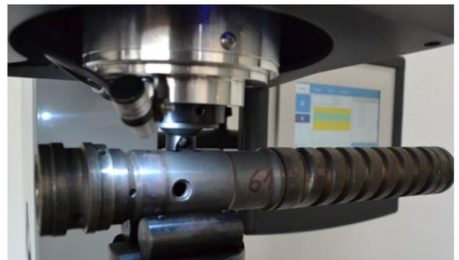
Cylindron Anvil for cylindrical parts from 50mm to 203mm in
