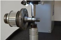
Clamping device with auto-stop function, clamping force ca. 60kgf (130lbs)
