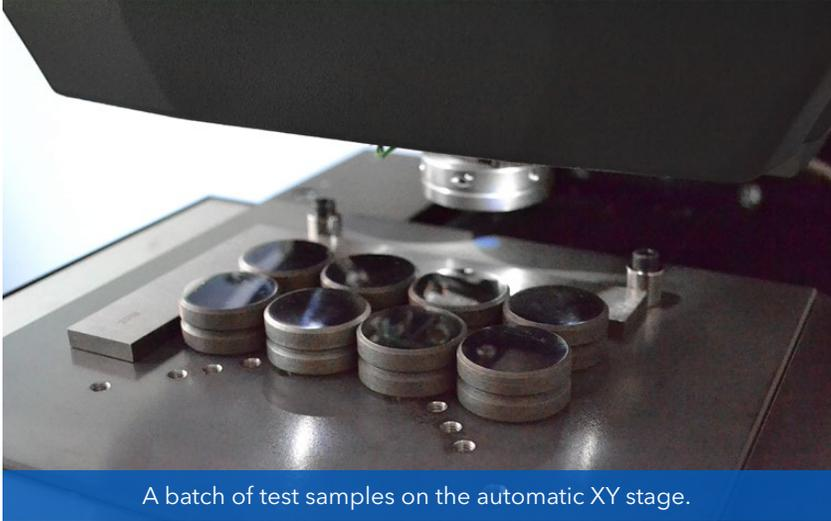
A batch of test samples on the automatic XY stage.
