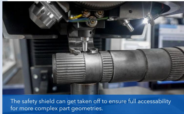
The safety shield can get taken off to ensure full accessibility for more complex part geometries.
