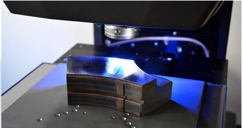
Large piece of casting to perform HBW2.5/187.5 Brinell hardness testing fully automatic around the contour.
