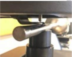
The unique clamping device for the UH4000 series hardness testers ensures that workpieces will be fixed properly during testing. The device is designed to adapt different types of clamping forks. Clamping width: 35mm [1.37in]
