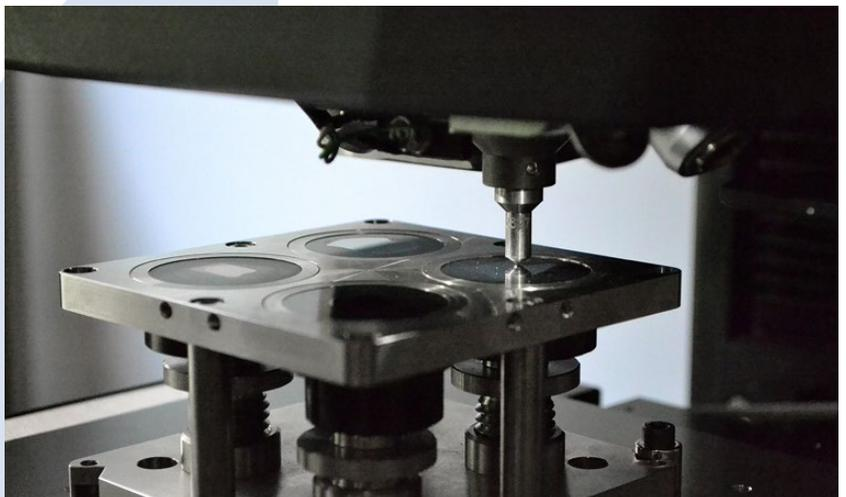
Mounted samples using a sample holder for multisample testing.
